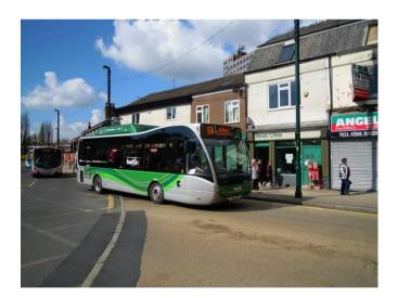
One of the new diesel electric hybrids passes through Eccles recently. Setting off using the electric motor gives them a quiet and rapid acceleration.
