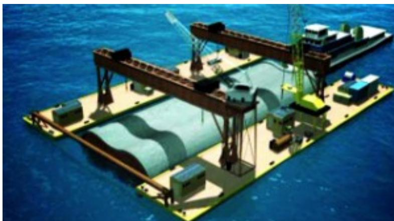
*A computer graphic illustrating the method of construction of the sea bed section of the Marmaray tunnel on the Eccles to Beijing Intercontinental Railway.*
